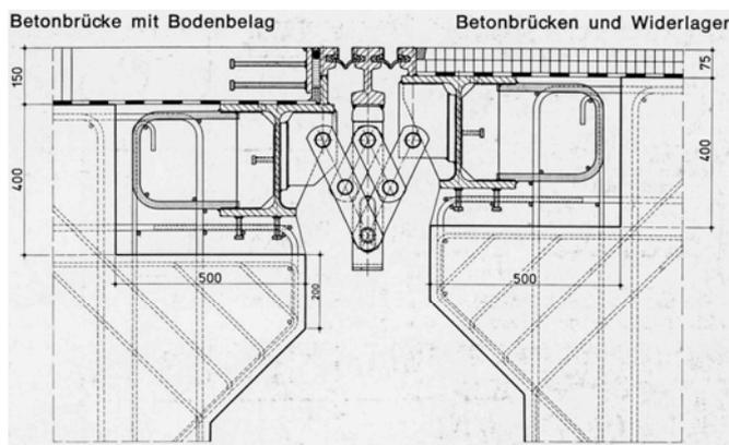
Fig.3. The rubber profiles and the small stones between the bearing rails [2]
